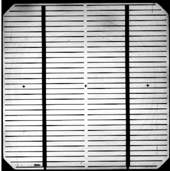
Fig. 11. Analyses of output local current of the sample no. 3 by usage of focused LED diode with middle wavelength 430 nm (blue LED, T=297 K)
